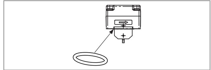
Fig. 27: Seal for metal fitting
