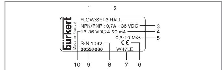
1. Measured value and type of the device
