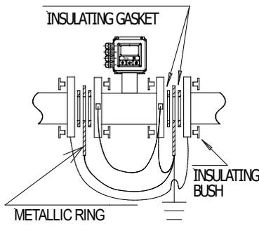
If the sensor must be install in the piping with a chatode protection, is necessary:
