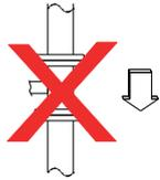
For vertical installations with descending flow direction contact the manufacturer
