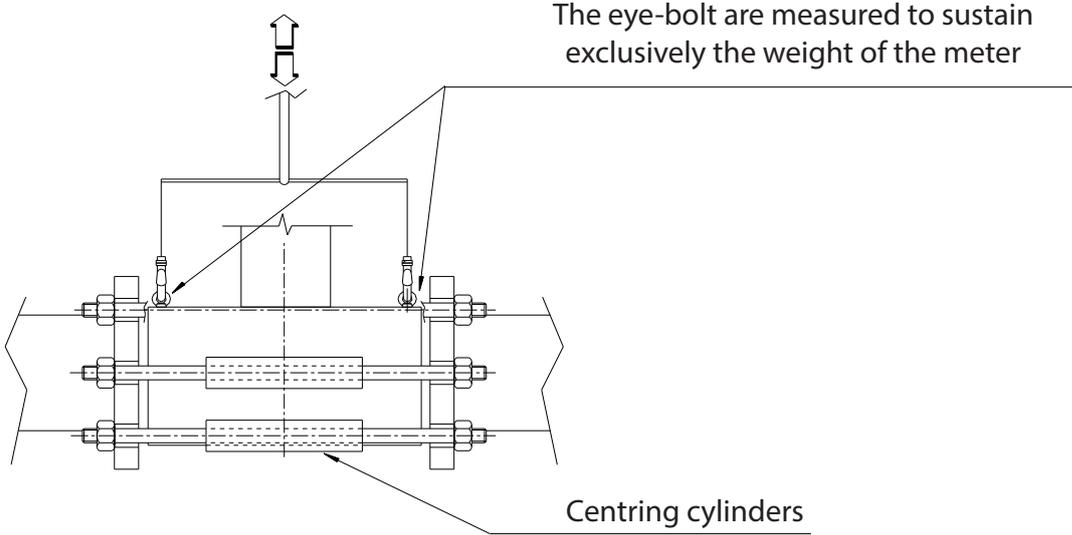
N.B.: For sensor S054 we recommed the use of centring cylinders
