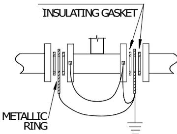
If the sensor has to be mounted on a pipe made of an insulating material is necessary:
