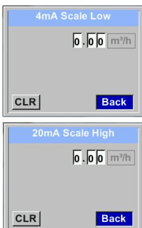
The scaling of the 4-20mA channel can be done automatically "Auto Range = on" or manual "AutoRange = off".
