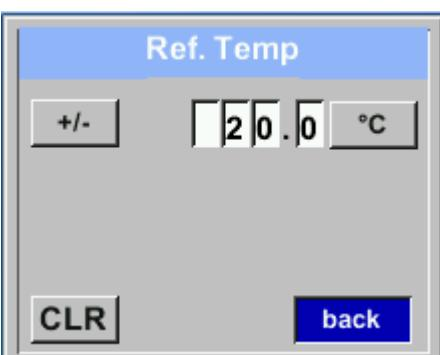
By pressing „△“ the position value is incremented by 1. Complete with “**OK**” and activate next number position.
