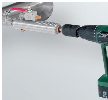
In case the system could not be shut down, means to be set depressurized, there could be used the spot drilling collar and drilling jig to drill through the ball valve.
