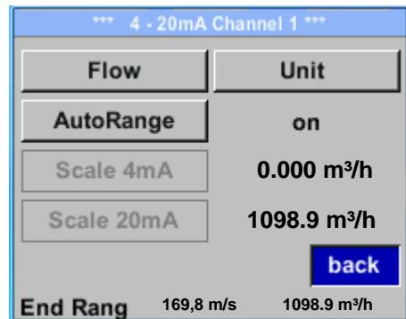
The 4-20 mA Analogue output of the Sensor Typ 8007 can be individually adjusted.
