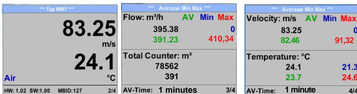
AV-Time ( Period for average value calculation) could be changed under [Sensor Setup.-Advanced- AV-Time](#)
