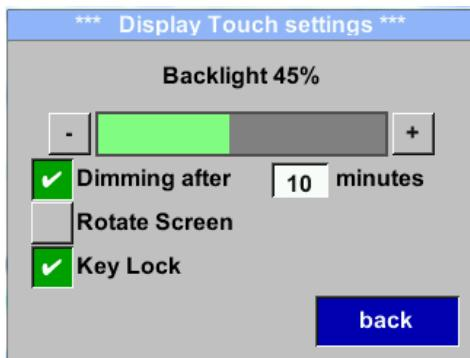
By activation of „**Key Lock**“ the operation of the sensor locked.
