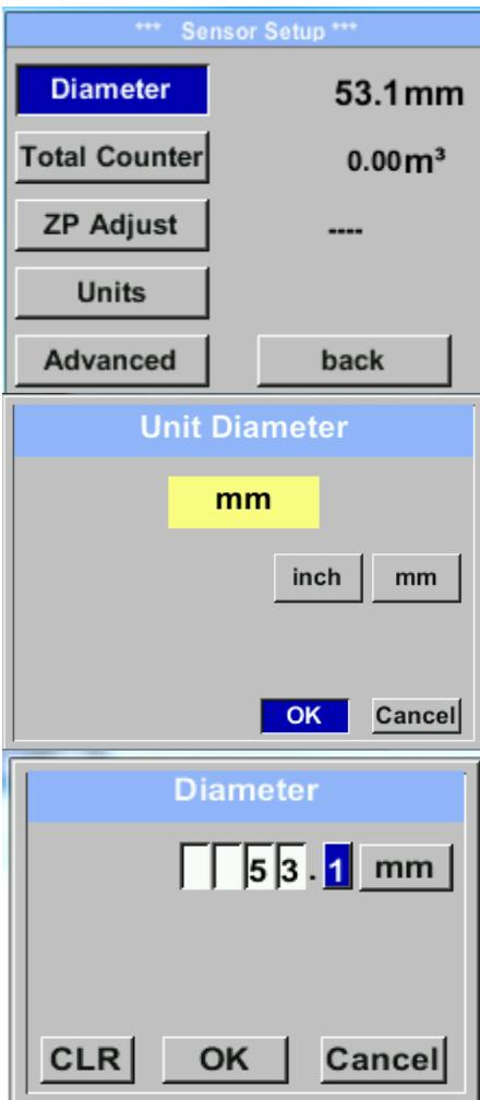
In order to change, e.g. the unit, first select by pressing key „ $\Delta$ “ the field “Units” and then key “OK”.
