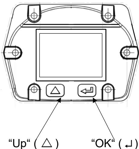
The operation of the Typ 8007 is done by the two capacitive key buttons Up ( $\triangle$ ) und Enter ( $\leftarrow$ )
