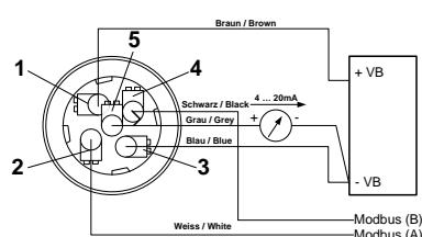
**Connector plug B (M12 - A-coding)**
