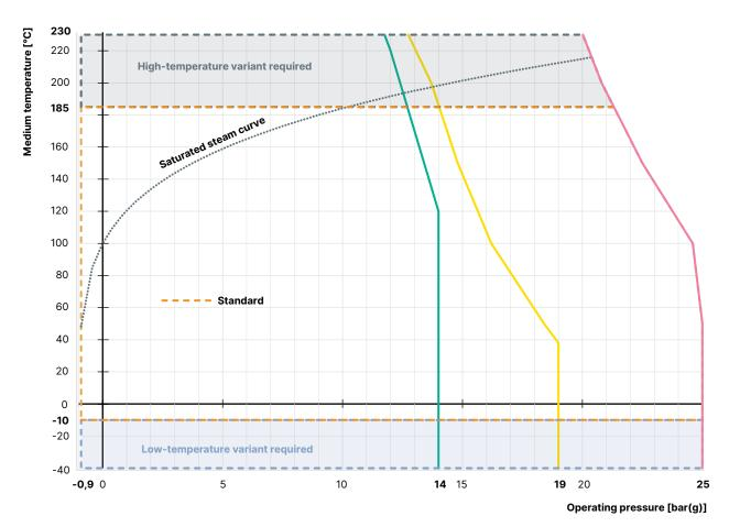
Operating limits for PN25 according to DIN EN 12516-1
