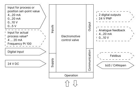
Note: Optional outputs are represented with a broken line
