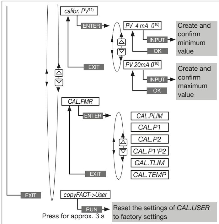
Fig. 21: Operating structure CAL.USER, changing the factory calibration 2
