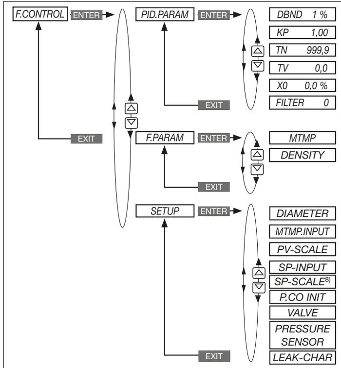
Fig. 17: Operating structure - basic settings for flow controller
