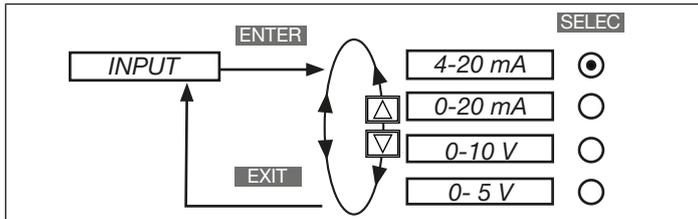
Fig. 16: Operating structure *INPUT* (select input signal)
