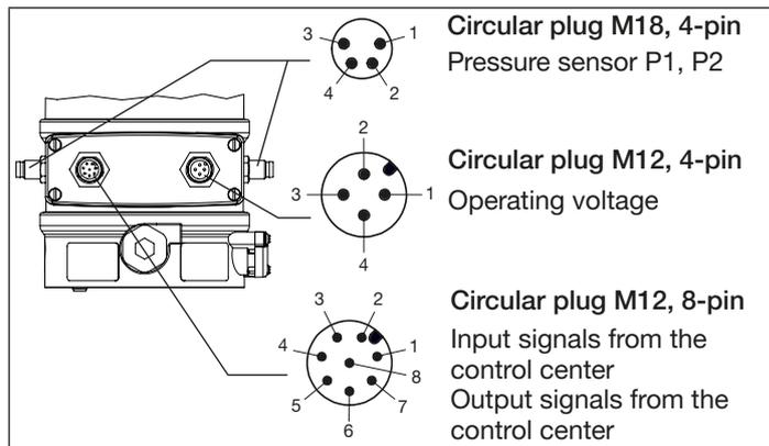
Fig. 13: Connection with 24 V DC circular plug-in connector
