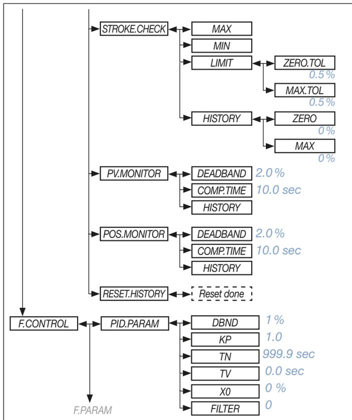
Fig. 38: Operating structure FMR – 15
