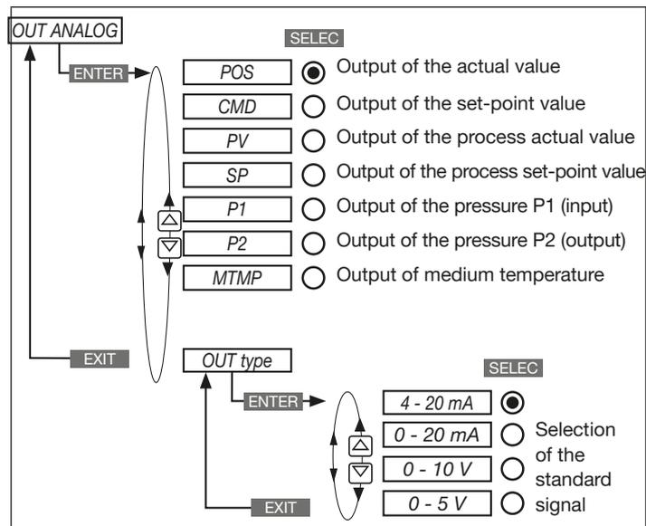
Fig. 22: Operating structure OUT ANALOG - analog output
