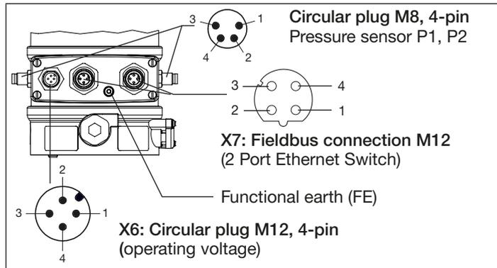
Fig. 15: Connection EtherNet/IP, PROFINET and Modbus TCP
