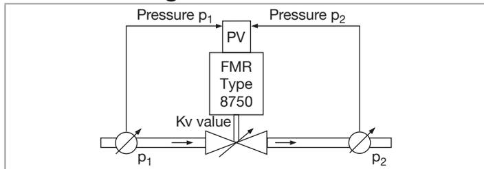
Fig. 2: Action diagram
