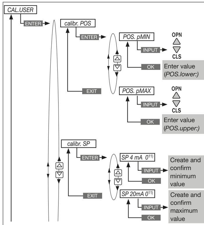
Fig. 20: Operating structure *CAL.USER*, changing the factory calibration 1
