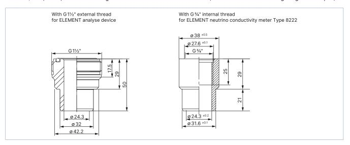
In PVC-U / FKM, EPDM, to stick on T-fitting d50 × 32 to d110 × 32 with solvent socket (variable d: see note at the beginning of the chapter)
